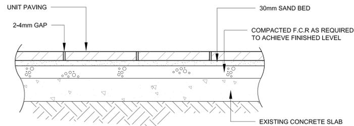
9 UNIT PAVING OVER CONCRETE SLAB
